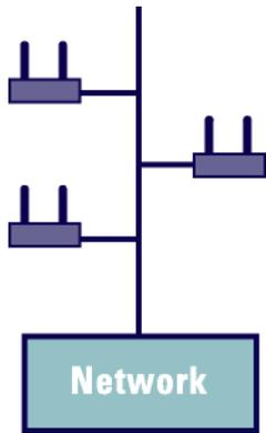
**Point products:** *Access point products must be carefully placed and manually configured, don't offer wireless intelligence and are isolated islands within the network.*
