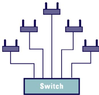
**WLAN (switches):** *Centralized WLAN's require stepwise growth, can't tune for performance, and if the switch fails, all coverage is lost.*
